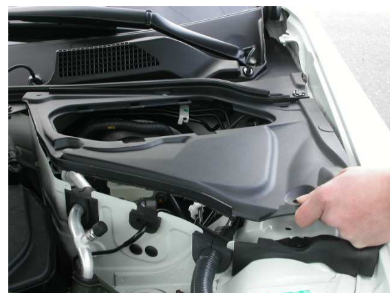
6.A. Place driver's side battery cover in place. Start with the top edge closest to the firewall.
