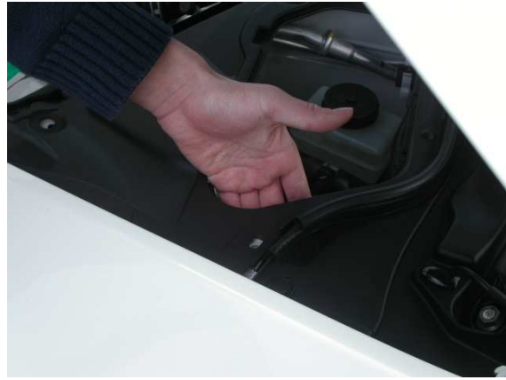
7.A. To secure the hole in the upper right portion, place a rivet clip through the hole and into the hole running flush from the bracket. Hold onto the bracket with your hand to secure it in place, while inserting the rivet cap.
