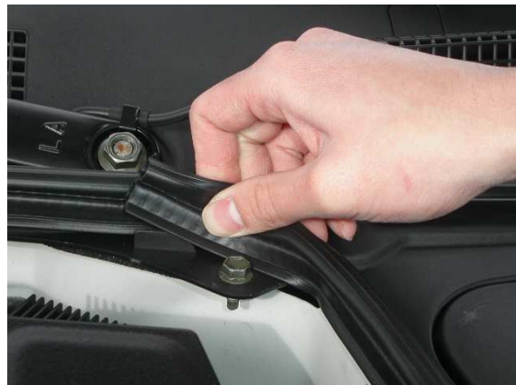
9.B. Then finish replacing the weather stripping at the top.
