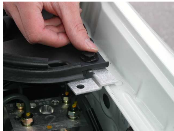
4. Replace rivet cap that was removed in Step 2 to secure bracket.
