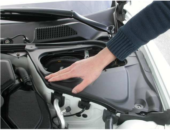
6.B. Then place the bottom half of the cover to make a snug fit.
