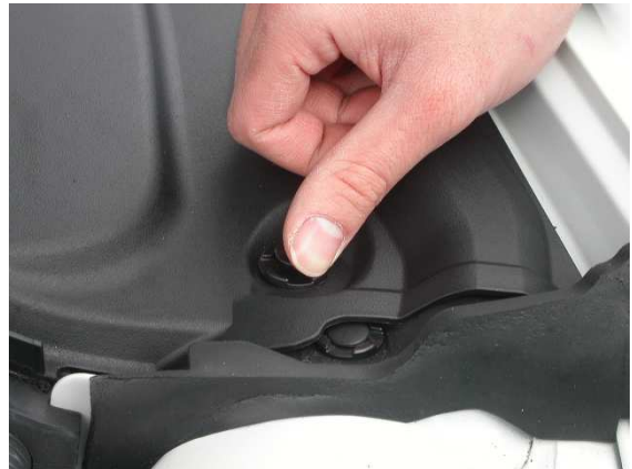
8. Place a rivet cap to secure the hole in the lower right portion of the battery cover. This hole was created via Step 1.
