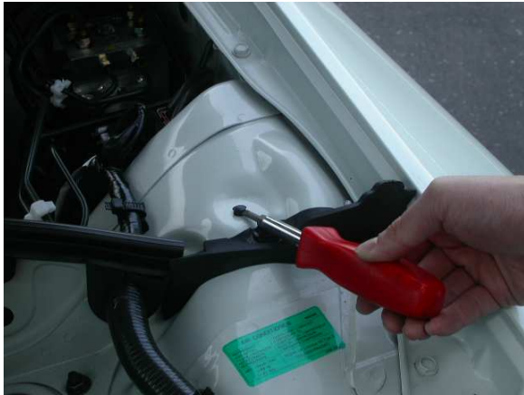
1. Remove hole cover by carefully prying out with a flathead screwdriver.
