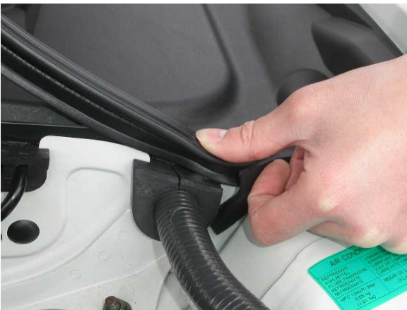
9.A. Replace stock weather stripping starting from the bottom. Make sure that the stripping runs flush with the battery cover.
