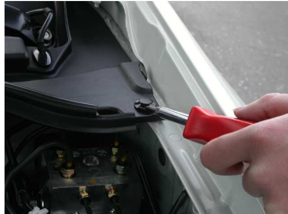
2. Remove rivet cap from upper right hand corner of the compartment.
