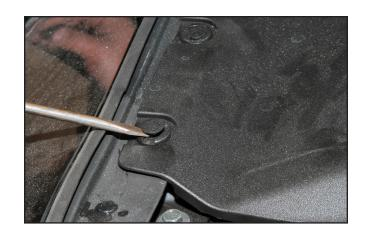
3. REMOVE STOCK AIR BOXES BY UNDOING THE (2) 10MM PHILLIPS BOLTS AND THE 8MM HOSE CLAMP ON THE TURBOCHARGER (PICTURED ON RIGHT IS THE "HIDDEN" 8MM HOSE CLAMP).
