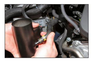
7. ATTACH THE MAF SENSOR HOUSING
