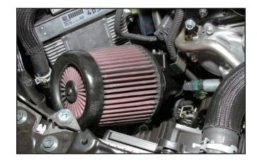
10A. REMOVE THE STEEL SLEEVE AND RUBBER VIBRATION DAMPERS FROM THE STOCK AIR BOXES AND REPLACE THEM ONTO THE FILTER SHROUDS. TO REMOVE, PRESS THE STEEL SLEEVE OUT OF THE GROMMET, THEN REMOVE THE GROMMET FROM THE AIR BOX. REINSTALL IN REVERSE ORDER.
