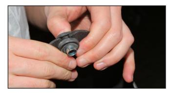
10B. MOUNT THE URETHANE FILTER SHROUDS TO THE BODY USING THE TWO MOUNTING HOLES.
