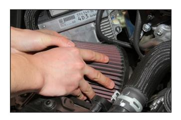
9. ENSURE THERE ARE NO CLEARANCE/ RUBBING ISSUES AND THEN TIGHTEN ALL OF THE HOSE CLAMPS.
