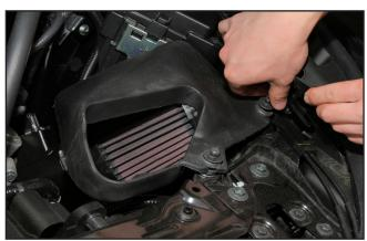
11. ATTACH STOCK AIR DIVERSION PANEL TO THE FILTER SHROUDS AND SECURE IT WITH THE 6 FACTORY CLIPS
