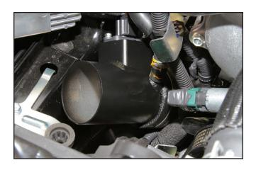
8. ATTACH THE AIR FILTER TO MAF FLANGE.
