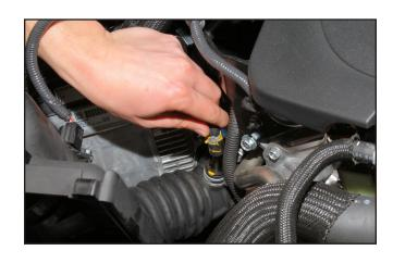
5. USING A PHILLIPS SCREWDRIVER, CAREFULLY REMOVE THE MAF SENSOR FROM THE STOCK AIR BOXES AND INSTALL THEM ON THE MAF SENSOR HOUSINGS INCLUDED WITH THE STILLEN INTAKE KIT BY MATCHING THE ARROWS. THE SENSORS WILL ONLY FIT IN THE FLANGE ONE WAY.
