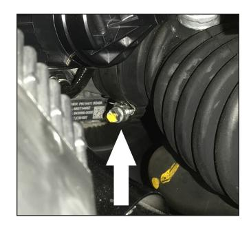
4. UNPLUG BOTH MASS AIR FLOW (MAF) SENSOR CONNECTORS AND THE POSITIVE CRANKCASE VENTILATION (PCV) HOSE (PASSENGER SIDE ONLY)
