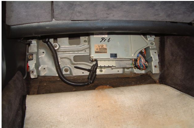
Figure 2 – Factory ECU Mounting Location with cover removed
