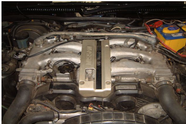
Figure 6 – Internal MAP sensor vacuum line installed
