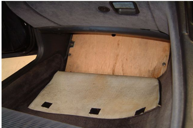
Figure 1 – Left hand footwell showing ECU cover
