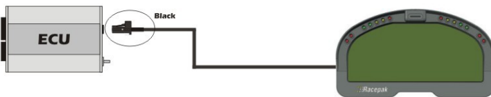
Figure 9 – Haltech ECU connected to a Racepak Dash
